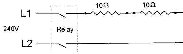
The working voltage is divided across each component in a series circuit. In the figure above if both resistors (heating elements) have the same resistance in ohms then the voltage would be consumed evenly between them. Specifically, if the applied voltage is 240 then each element would behave like a 120v element ( $240v / 2 \text{ elements} = 120\text{volts/element}$ ). Elements would be designed to operate on 120v instead of 240v when there are 2 elements in a series circuit.
