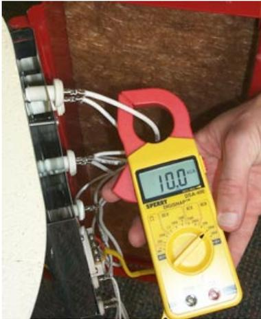
*Testing Amperage at Feeder Wires*
