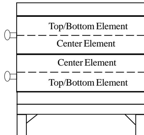
**PLEASE NOTE:** The elements for all other kiln models are the same from top to bottom for each model. This includes models 609, 614, 714, KS818, KS818P, KS818WR, KS818PWR, 181, 180, 145, 183, 185, the Pinto, and Octagon Fuser. Element positioning is not effected by phase or brick size.
