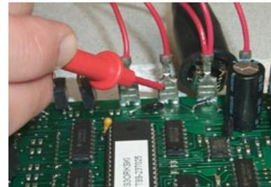
*Measuring Controller Voltage*
