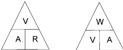
These 2 equation triangles are helpful in determining the proper formula to use. For example: by placing your finger over "R" in triangle 1 the remaining symbols express the formula for calculating "R", V/A.
