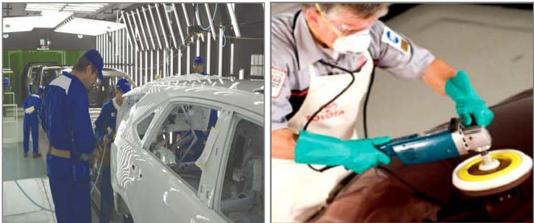
EXAMPLE IMAGES OF TOPCOAT ULTRA-FINE SANDING AND POLISHING TO REMOVE PROCESS INTRUSION DIRT NIBS - FACTORY AND BODY SHOP
