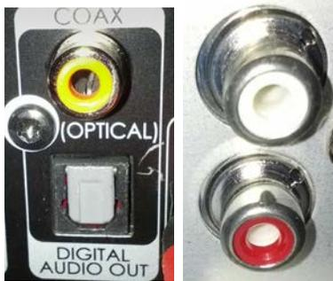
On the top left are digital connectors using RCA Digital Audio COAX. On the bottom left, Optical Digital Audio. The connectors on the right are standard RCA Phono Audio connectors, such as have been used on stereos for many years. Many televisions will also have a headphone jack, such as you would find on a Smartphone or iPod.
