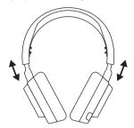
2 Change the position of the *Elastic Headband (1)* on one or both sides to achieve the desired tension and flex.
